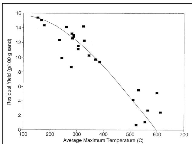
**FIGURE 5: Hydrocarbon remaining on core following ramped temperature oxidation of Athabasca Oil Sands bitumen.**
