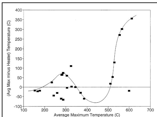
**FIGURE 4: Energy generation resulting from ramped temperature oxidation of Athabasca Oil Sands bitumen.**
